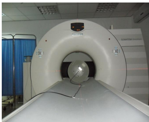
Figure 1: Experimental set-up for the measurement of CTDI with the dose profiler probe [Field work, 2016]
