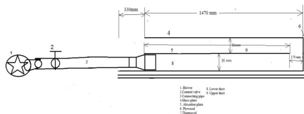
**Figure 1.** Schematic diagram of Experimental setup
