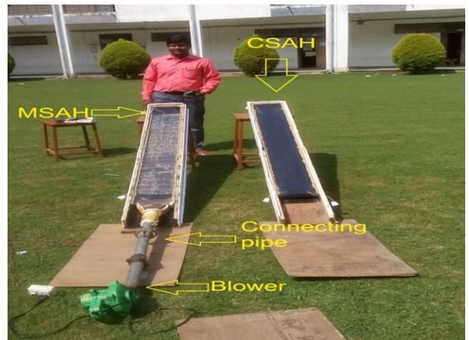
Figure 2. Pictorial view of experimental setup
