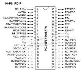
Figure 3. PIC16F877A Pin Diagram
