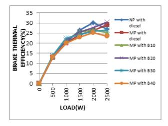
Figure 9. Load VS Brake Thermal Efficiency
