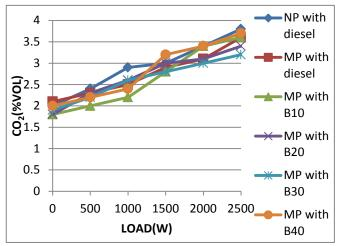
Figure 12. Load vs CO<sub>2</sub>Emissions
