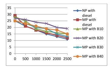
Figure 11. Load vs HC Emissions
