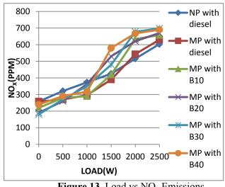
Figure 13. Load vs NO<sub>x</sub> Emissions
