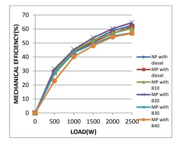
Figure 8. Load vs Mechanical Efficiency
