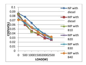
Figure 10. Load vs CO Emissions
