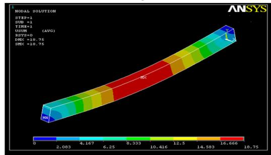
Figure 8 Deflected profile of uncracked laminated beam ABP2 at yield stage
