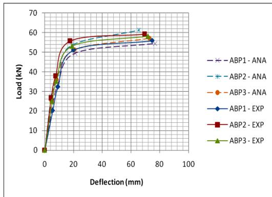
Figure 11 Comparison of analytical and experimental load-deflection response of uncracked laminated beams
