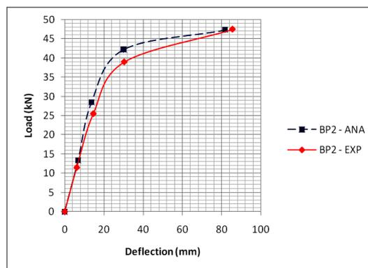
Figure 10 Comparison of analytical and experimental load-deflection response of perfect beam
