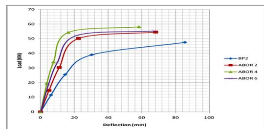
Figure 5 Load-deflection behaviour of precracked rehabilitated beams
