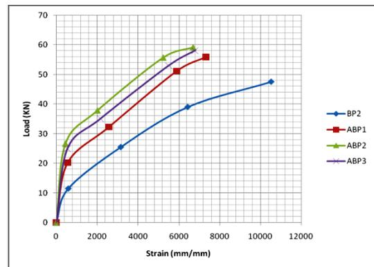
Figure 4 Load-rebar strain profile for perfect and uncracked laminated beams
