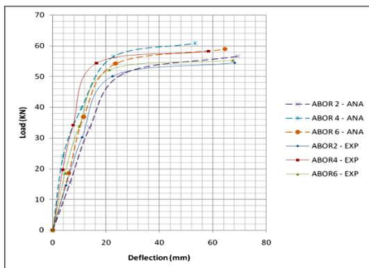
Figure 12 Comparison of analytical and experimental load-deflection behaviour of precracked rehabilitated beams
