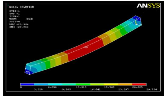
Figure 7 Deflected profile of perfect beam BP2 at yield stage
