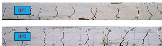
Figure 2 Crack pattern and failure mode of perfect beams
