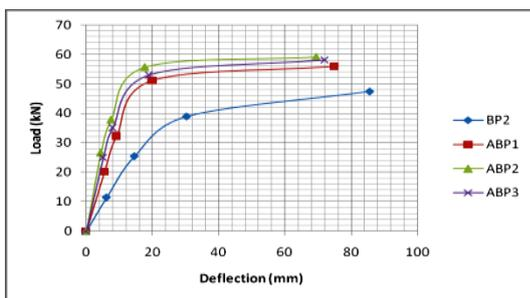
Figure 3 Load-deflection behaviour of uncracked laminated beams
