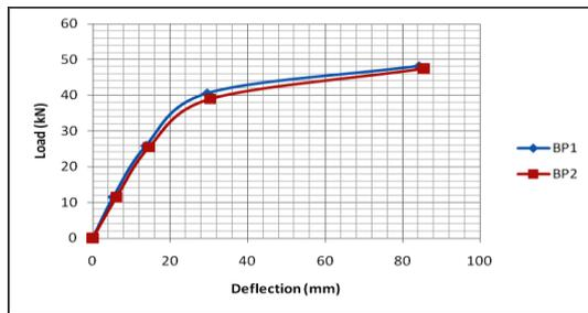
Figure 1 Load-deflection curve for perfect beams
