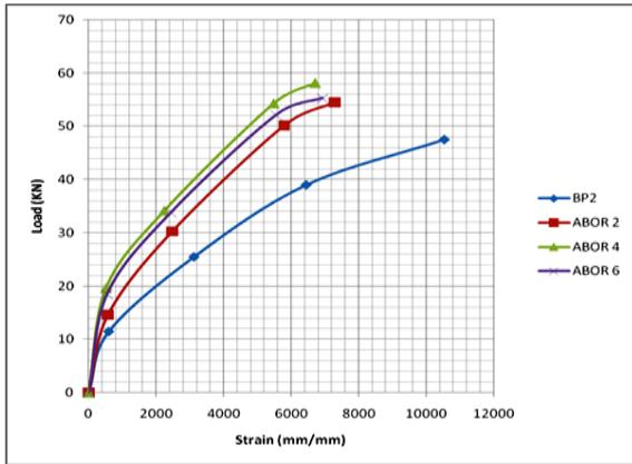
Figure 6 Load-rebar strain profile for perfect and precracked rehabilitated beams
