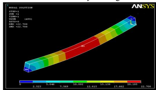
Figure 9 Deflected profile of precracked rehabilitated beam ABOR4 at yield stage
