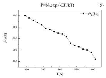
**Figure 1.** The variation of thermoelectric power with T for  $W_{0.90}$ Se2 single crystals
