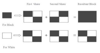
Figure 3: Encryption Rules Example
