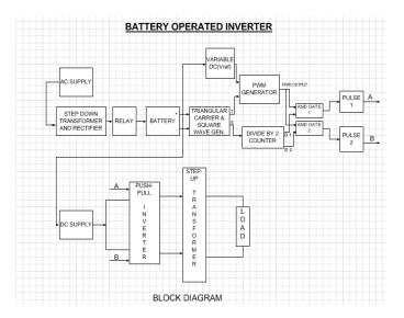
The ac supply is given to a step down transformer followed by a rectifier unit. The dc obtained is given to the relay COIL .The relay has 2 CO contacts. As per the relay operation, when ac supply is ON the battery is charged and supply is given to load. When the ac supply is OFF the battery gives supply to the inverter circuit and the output of it is given to the step up transformer and then fed to load.
