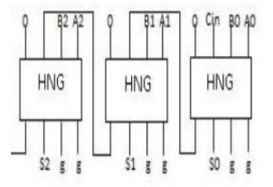
Figure 8. Ripple carry adder
