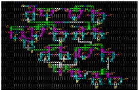
Figure 16. QCA layout for the Logic unit
