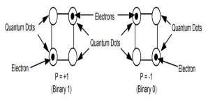
Figure 1. QCA Polarization cells with +1 for logic 1 and -1 for logic 0.
