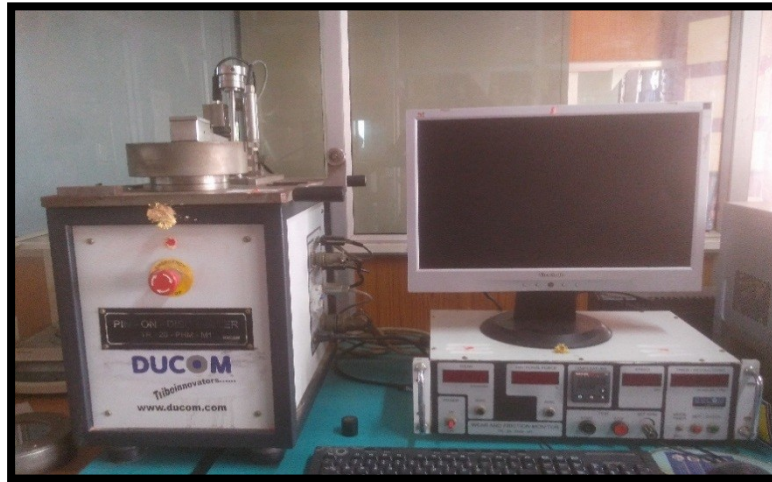
Figure 3: Pin on Disc wear test machine
