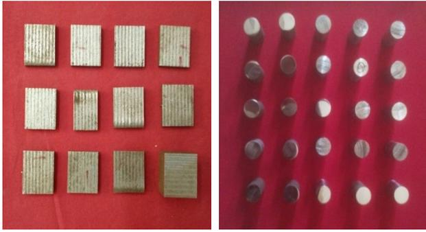
Figure 2. Laser Hardfaced samples
