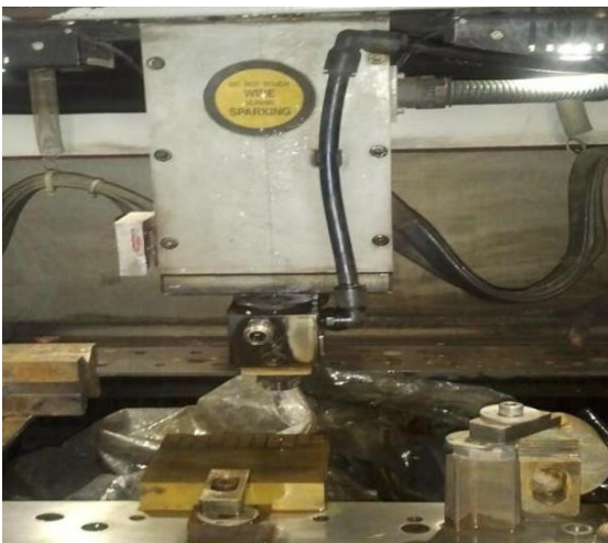
Figure 1. Work piece Mounted on WEDM
