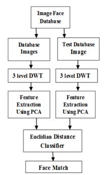
Figure1: Proposal DWT based PCA Algorithm
