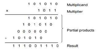
Figure 2. Example of array multiplier
