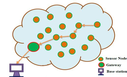
**Figure 1.** The schematic view of the wireless sensor network
