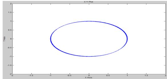
Figure 11. Stator flux trajectory curve Proposed.
