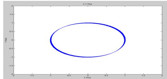
Figure 10. Stator flux trajectory curve existing
