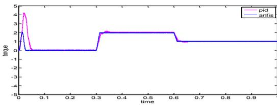
Figure 6. Torque response curve of Proposed and Extension.
