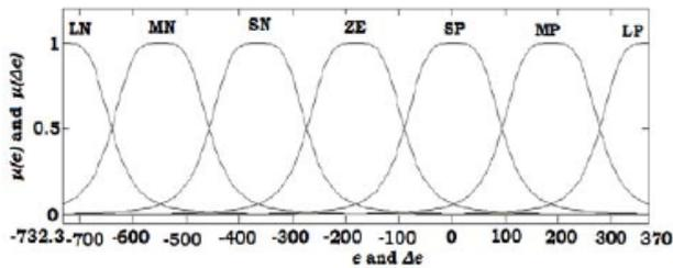
Figure 5. Membership functions for error and change in error.
