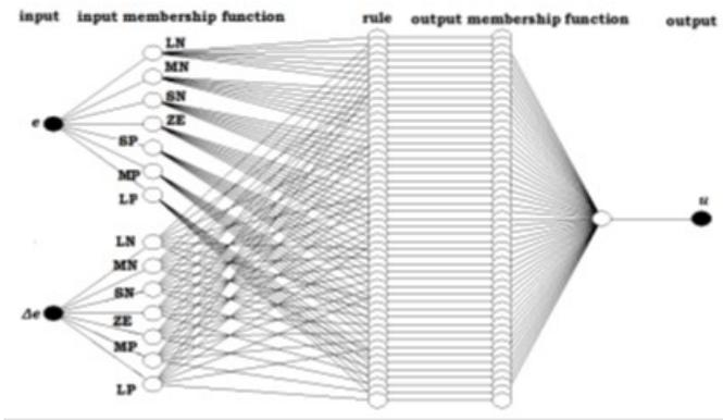
Figure 4. The network of ANFIS controller
