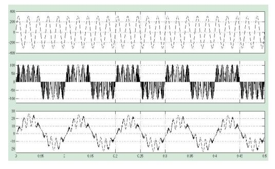
**Figure 12.**(a)Source Voltage(b)OutputVoltage(c)OutputcurrentWaveform ofSinglePhasetoSingle Phase CycloconverterWhen InputFrequencyisFiveTimesOutputFrequency
