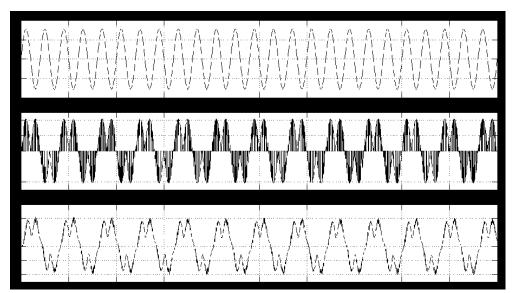
$\label{eq:Figure3.} Figure3. (a) SourceVoltage (b) Output Voltage (c) Output current Waveform of Single Phase to Single Phas$
