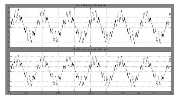
**Figure 10.**(a)MainWindingCurrent (b)AuxiliaryWinding Current Waveformof SinglePhase Induction Motor, When InputFrequencyto the CycloconverterisFourTimesOutputFrequency.
