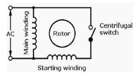
Figure2.Single-phasemotor- Resistancestart splitphasemotor
