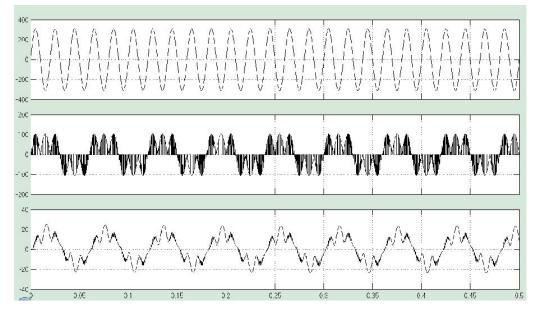
$Figure 6. (a) \\ Source \\ Voltage (b) \\ Output \\ Voltage (c) \\ Output \\ current \\ Waveform of \\ Single \\ Phase to \\ Phase to$
