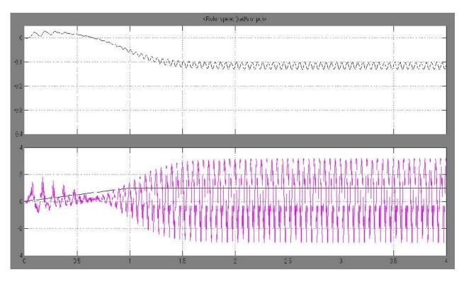
**Figure14.**(a)RotorSpeed(b)LoadandElectromagneticTorqueWaveformof SinglePhaseInduction Motor, When InputFrequencyto theCycloconverteris fiveTimesOutputFrequency.
