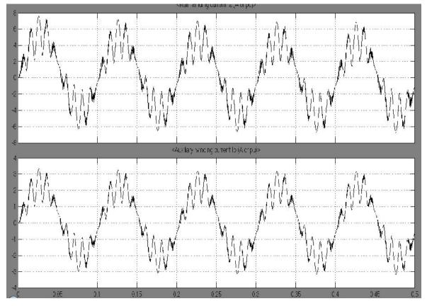
**Figure13.**(a)MainWindingCurrent (b)AuxiliaryWinding Current Waveformof SinglePhase Induction Motor, When InputFrequencyto the CycloconverterisFiveTimesOutputFrequency.
