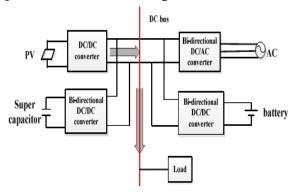
**Figure 8.** Power flow of mode I
