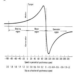
**Figure 11.** AC Induction Motor Speed-Torque Characteristic
