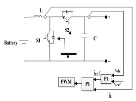
**Figure 4.** Control strategy of the bi-directional DC/DC converter
