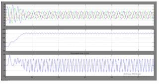
**Figure 17.** simulation wave form of DC microgrid with Induction Motor stator current, speed and electromagnetic torque
