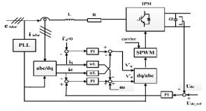
**Figure 5.** Control strategy of the bi-directional DC/AC converter
