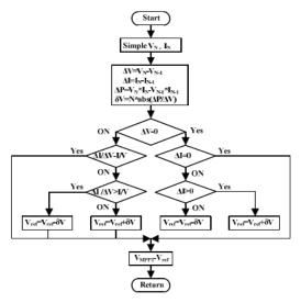
**Figure 3.** Flowchart of the variable step size INC MPPT algorithm
