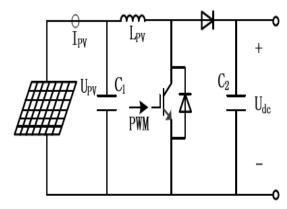
**Figure 2.** DC/DC converter of PV module with MPPT function
