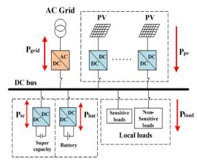
Figure 1. DC microgrid with hybrid storage system
