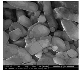
Figure 2. SEM image of the Ferrogel
