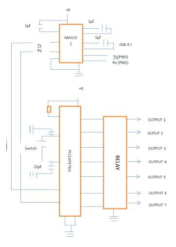
Figure 4: Main component circuit analysis
