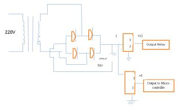
Figure 3: Power supply regulation circuit
