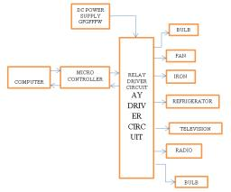
Figure.2: Block Diagram of the designed system
