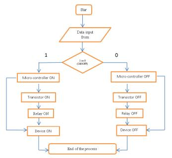
Figure 7: The flow chart of the designed system
