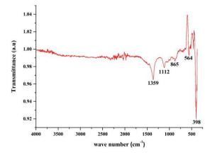
Figure 2. FTIR of pure ZnO nanoparticles
