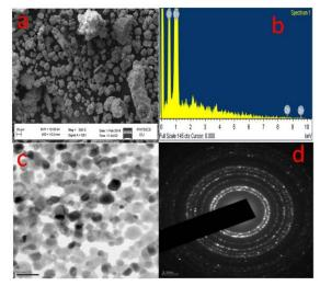
**Figure 3.** Micrograph of (a)SEM (b)EDS (c)TEM & (d)SAED of pure ZnO nanoparticles
