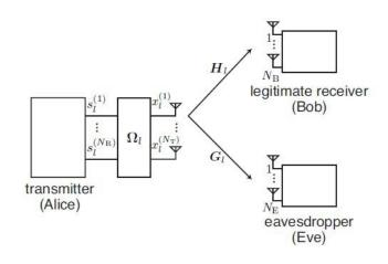
**Figure 5.** Mimo-Ofdm System With An Eavesdropper [32].
