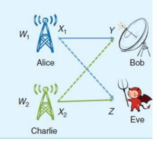
Figure 6. A Multiple Access Wiretap Channel
