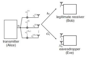
Figure 4. Miso-Ofdm System With An Eavesdropper
