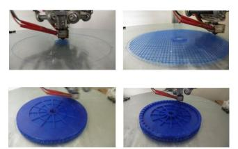
Figure 6. 3D Printing of Transmission Gear in 3D Printer
