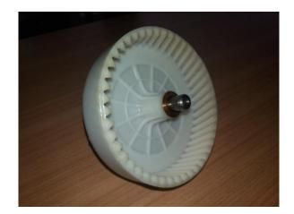
**Figure 2.** Helical Gear Made of Polymer Material using Injection Molding
