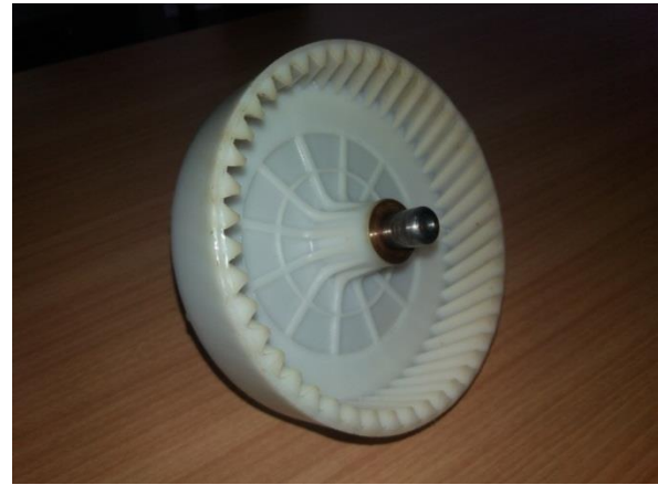
Figure 2. Transmission Gear Made of PLA
