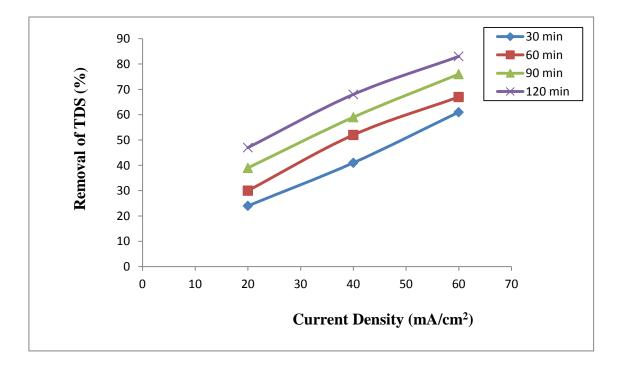
Fig. 4. Effect of current density on removal of total dissolved solids of Hindon water at 25.0  $^{\circ}$ C.
