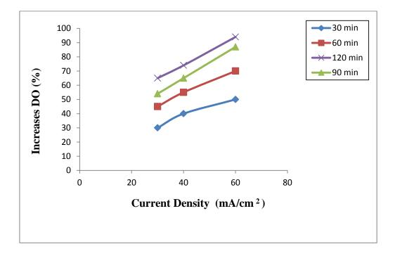
Fig. 7. Effect of current density on increasing of dissolved oxygen of Hindon water at 25.0  $^{\circ}$ C.
