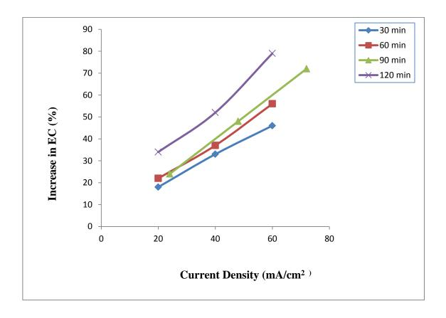
Fig. 8. Effect of current density on electrical conductivity of Hindon water at 25.0 °C.
