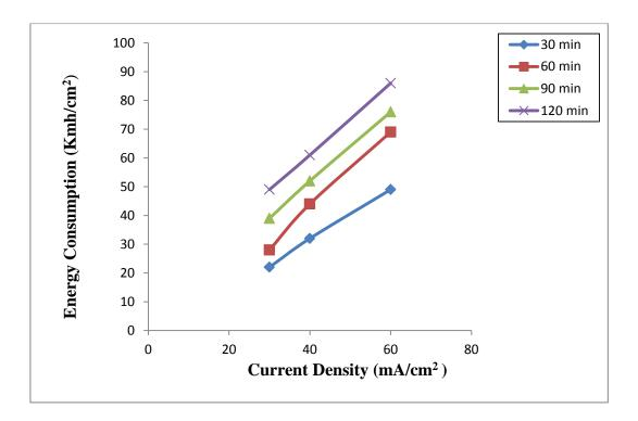
Fig. 12. Effect of current density on power consumption
