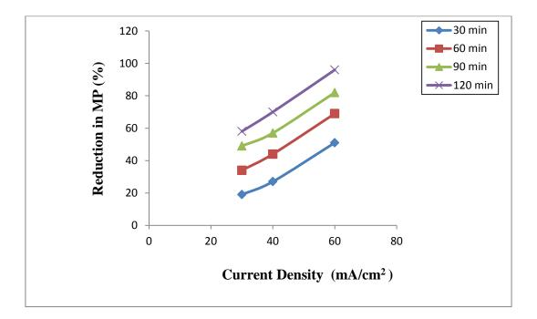
Fig. 9. Effect of current density on reduction of microbial population of Hindon water at 25.0 °C.
