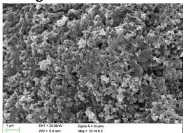
Figure. 5. SEM of Pure SnO<sub>2</sub>
