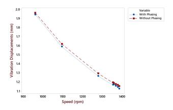
**Fig. 7** Comparison of vibration displacements vs speed of Gear Coupling sleeve.
