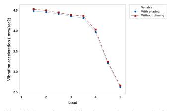
**Fig. 10** Comparison of vibration acceleration vs load of Gear Coupling sleeve.
