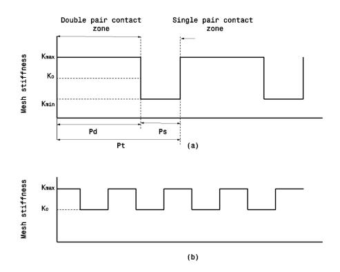
Fig. 2 Mesh stiffness (a) non-phased gear coupling (b) phased gear coupling
