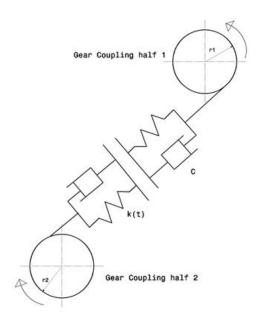
Fig. 1 Spur gear coupling model
