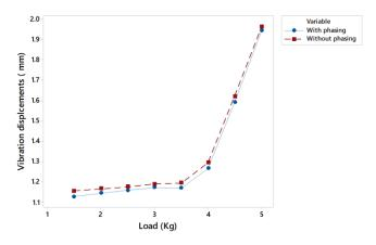
Fig. 9 Comparison of vibration displacements vs load of Gear Coupling sleeve.
