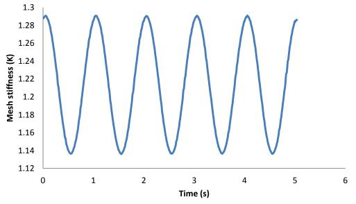
Fig. 3 Mesh stiffness variation for Non-phased gear coupling
