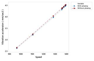
**Fig. 8** Comparison of vibration acceleration verses speed of Gear Coupling sleeve.
