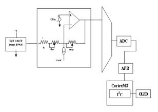
Figure 4: View of the circuit synthesized by adopting LiberoSoC on the chip A2F200M3F.
