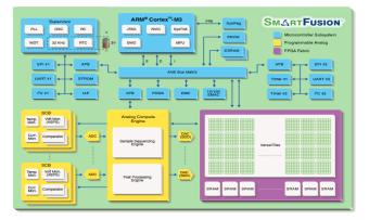
Figure 2: Architecture of Smart Fusion device A2F200M3F
