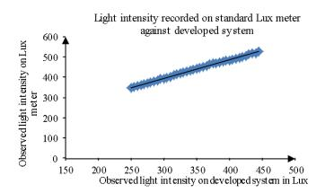
Figure 8: The plot of light intensity observed on developed system and Lux meter.
