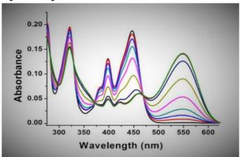
Figure 1. Absorption spectra of Probe (10  $\mu$ M) with 2 mM surfactant after addition of various concentrations of PhSH (0–100  $\mu$ M) at room temperature Three distinct absorbance peaks are observed 320 , 390, 445 nm after exposing Probe + CTAB with different conc of thiol will give rise to new absorbace peak at 550 appears due to formation NO $\rho$ f anionic chromophore. The color of the solution changes from colourless to pale red, indicating colorimetric detection of thiols
