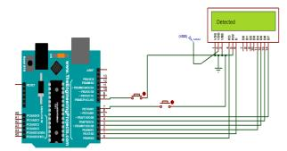
Figure 8. LCD interfacing view when NFC is successfully detected
