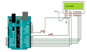
**Figure 9.** LCD interfacing view when NFC Detection Fail
