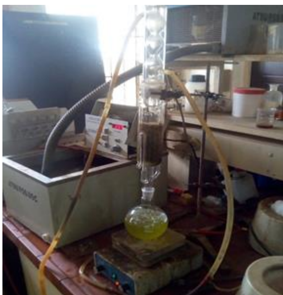
Plate 1. Soxhlet extractor set-up
