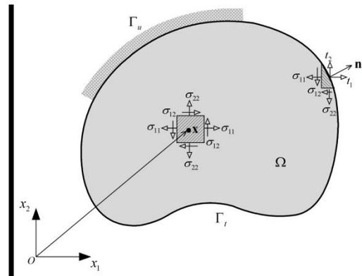
Figure 3. Schematic diagram for plane elastic problems
