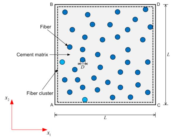
**Figure 1.** Schematic representation of regularly and randomly clustered fibers within the cement matrix
