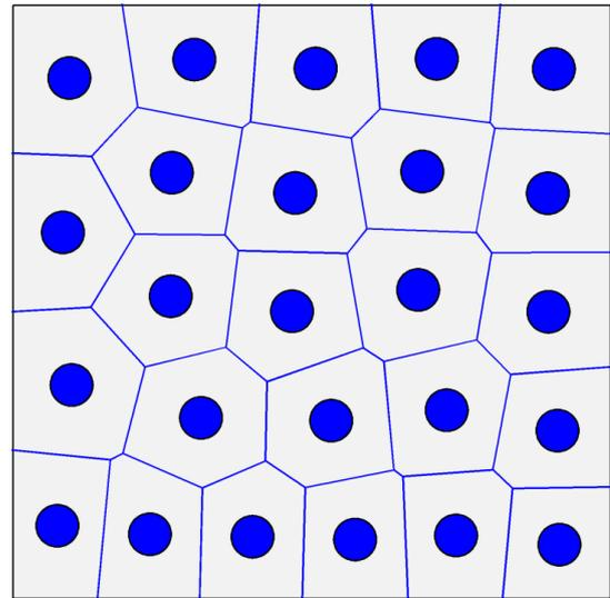
**Figure 2.** Schematic diagram of n-sided Voronoi fiber/matrix elements for the case of a random cluster
