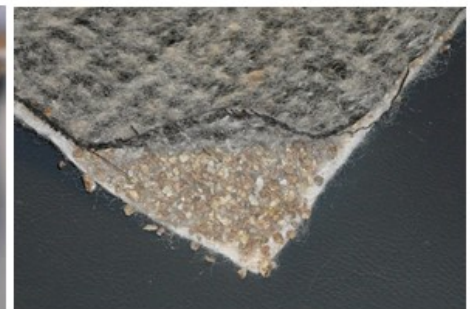
Figure 6. Geosynthetic Clay Liner
