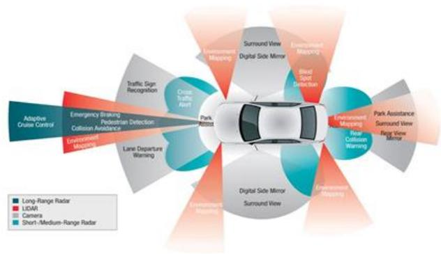
Figure 1. A visual representation of sensor fusion
