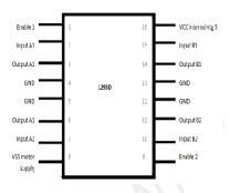
**Figure 4.** Pin configuration of L293DMotor driver IC **Logic used,**
