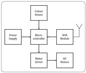
Figure 2. Receiver module
