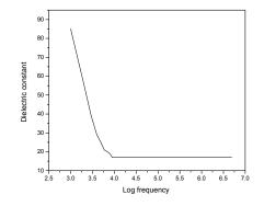
**Figure 5.** Dielectric constant of silver nitrate doped Zinc pottasium phosphate hexahydrate single crystal
