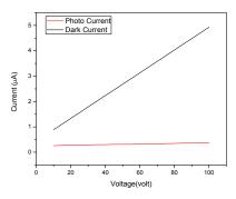
**Figure 2.** Photoconductivity of silver nitrate doped Zinc potassium phosphate hexahydrate
