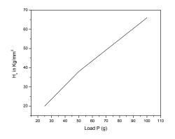
**Figure 4.** Microhardness of silver nitrate doped Zinc potassium phosphate hexahydrate single crystal
