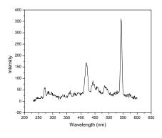
**Figure 1.** Photoluminescence of silver nitrate doped Zinc pottasium phosphate hexahydrate
