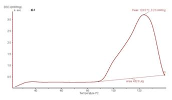
Figure 3. Differential scanning calorimetry (DSC) of silver nitrate doped Zinc potassium phosphate hexahydrate
