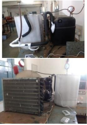
Figure 1. Experimental investigation of the refrigeration setup
