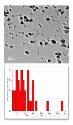
**Figure 3.** SEM and TEM images of synthesized silver naoparticles from *Coleus vettiveroids* aqueous leaf extract
