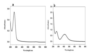
**Figure 4.** UV-Visible absorbance spectra of prepared (a) soap (b) soap impregnated with AgNPs.
