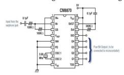
Figure 2. Dtmf Decoder 8870 Ic
