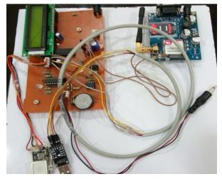
In this project we design two system, one is IVRS system and biometric fingerprint sensor based attendance system with notification SMS to parents using GSM.
