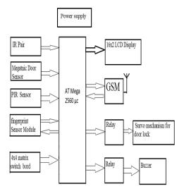
Figure 1. Block diagram of system. System Description -
