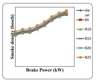
**Figure 4.** Variation of smoke density with power output
