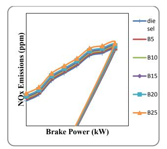
Figure 7. Variation of NOx emissions with power output
