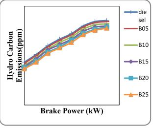
**Figure 5.** variations of hydrocarbon emissions with power output
