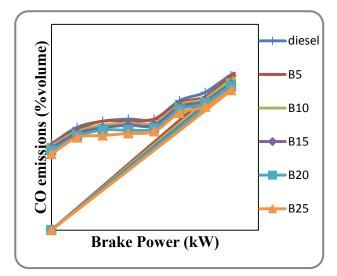
Figure 6. Variation of CO Emissions with Power output
