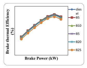
**Figure 1.** Variation of Brake thermal Efficiency with power output
