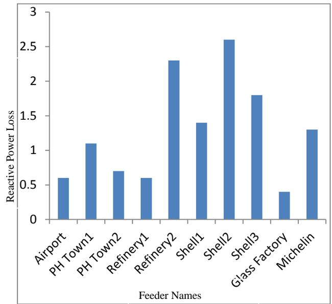
**Figure 9:** Reactive Power Loss before Tap changing for Port Harcourt distribution system
