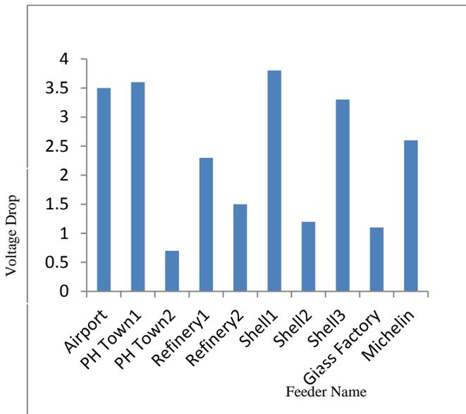
**Figure 7:** Voltage Drop before Tap changing for Port Harcourt distribution system
