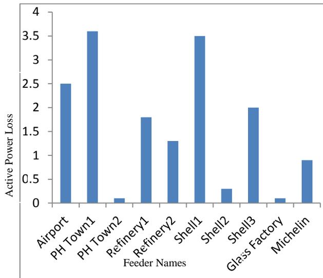
**Figure 11:** Active Power Loss after Tap changing for Port Harcourt distribution system
