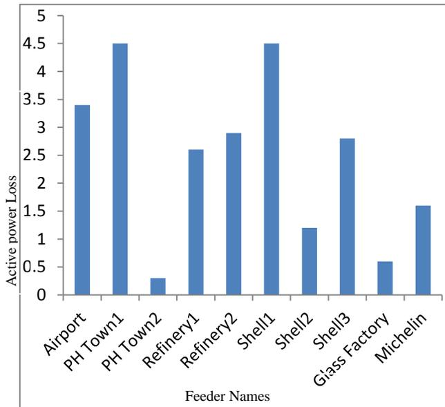
**Figure 8:** Active Power Loss before Tap changing for Port Harcourt distribution system
