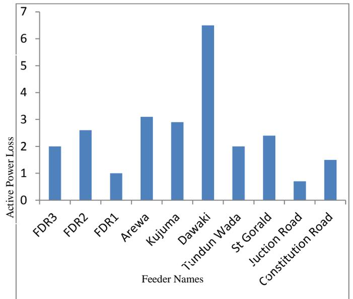
**Figure 5:** Active Power Loss after Tap changing for Kaduna distribution system
