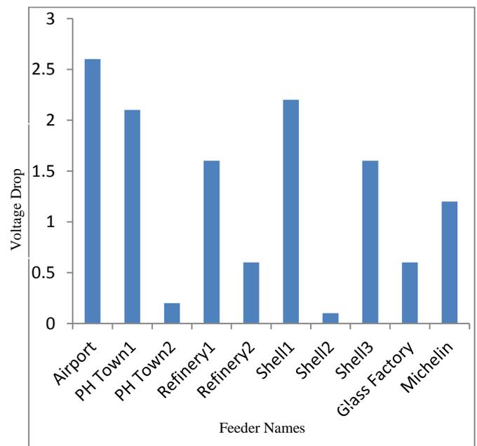
**Figure 10:** Voltage Drop after Tap changing for Port Harcourt distribution system
