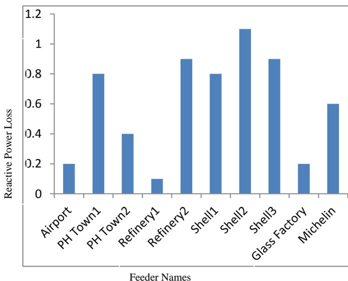
**Figure 12:** Reactive Power Loss after Tap changing for Port Harcourt distribution system.
