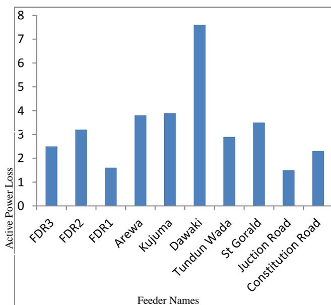
**Figure 2:** Active Power Loss before Tap changing for Kaduna distribution system
