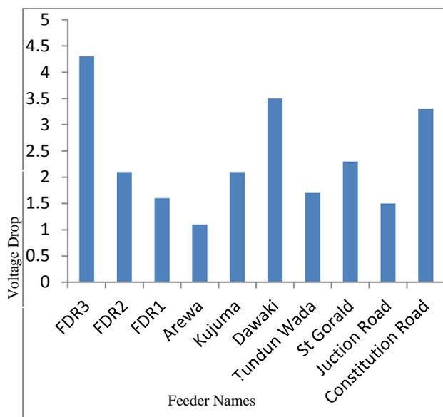
**Figure 1:** Voltage Drop before Tap changing for Kaduna distribution system
