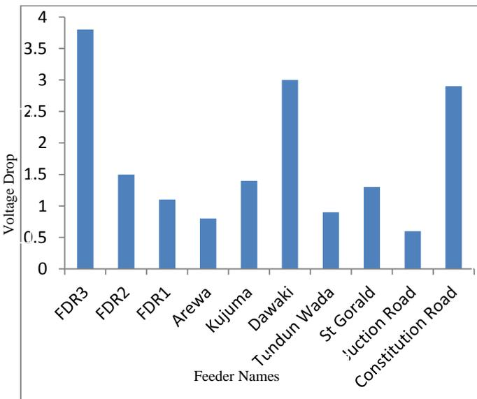
**Figure 4:** Voltage Drop after Tap changing for Kaduna distribution system
