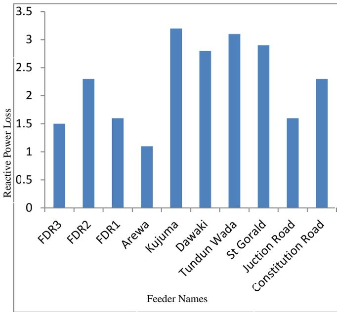
**Figure 3:** Reactive Power Loss before Tap changing for Kaduna distribution system
