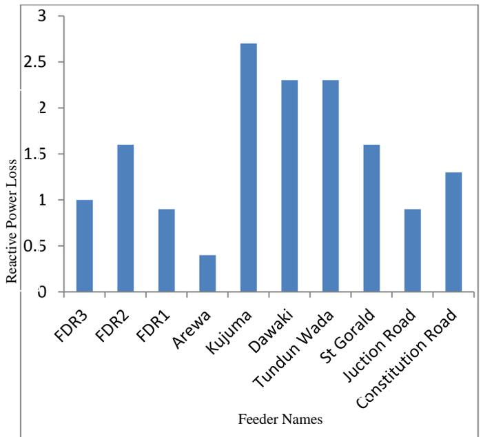
**Figure 6:** Reactive Power Loss after Tap changing for Kaduna distribution system
