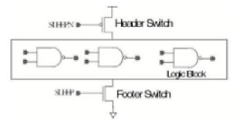
Figure 2: MTCMOS Circuit
