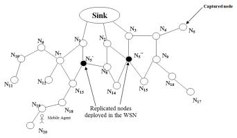
Figure 2 : Wireless Sensor Network randomly deployed in an area of interest
