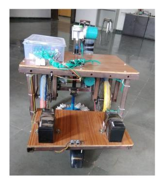
Figure 6. Hardware Model of Smart Floor Cleaner
