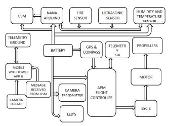
Fig: Block Diagram of the Project
