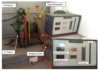
Figure 1: Engines with Control Panel
