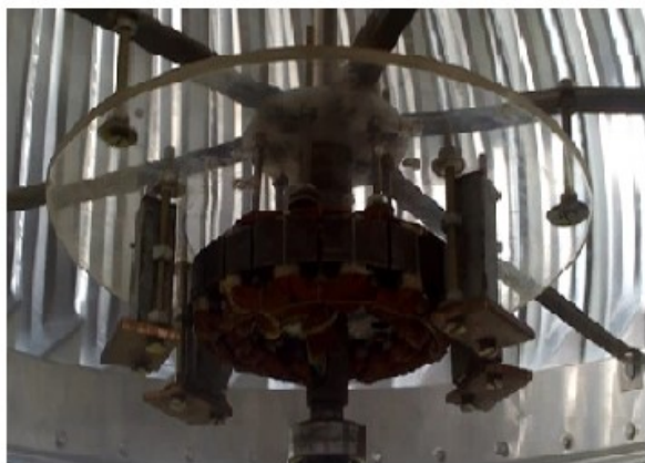
Fig. 7: Generator developed fitted to RTV frame.
