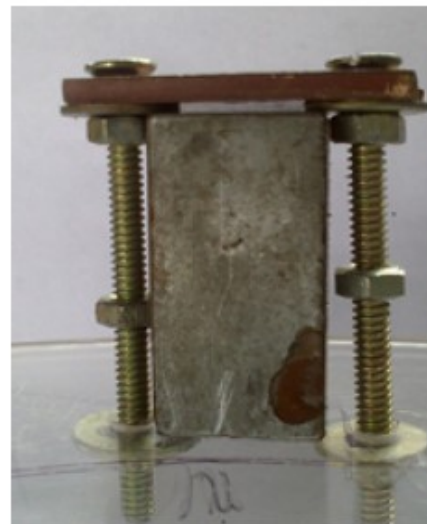
Fig. 5: Magnet bolted to the rotor frame
