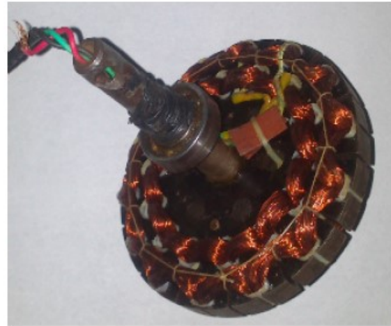
Fig. 3: Newly wounded core of the generator
