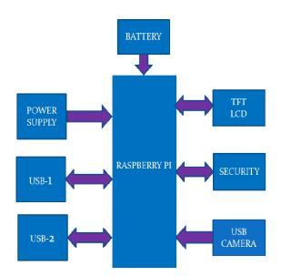
Figure 1. Block diagram of the project
