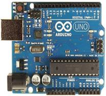
Figure 2. Arduino Board
